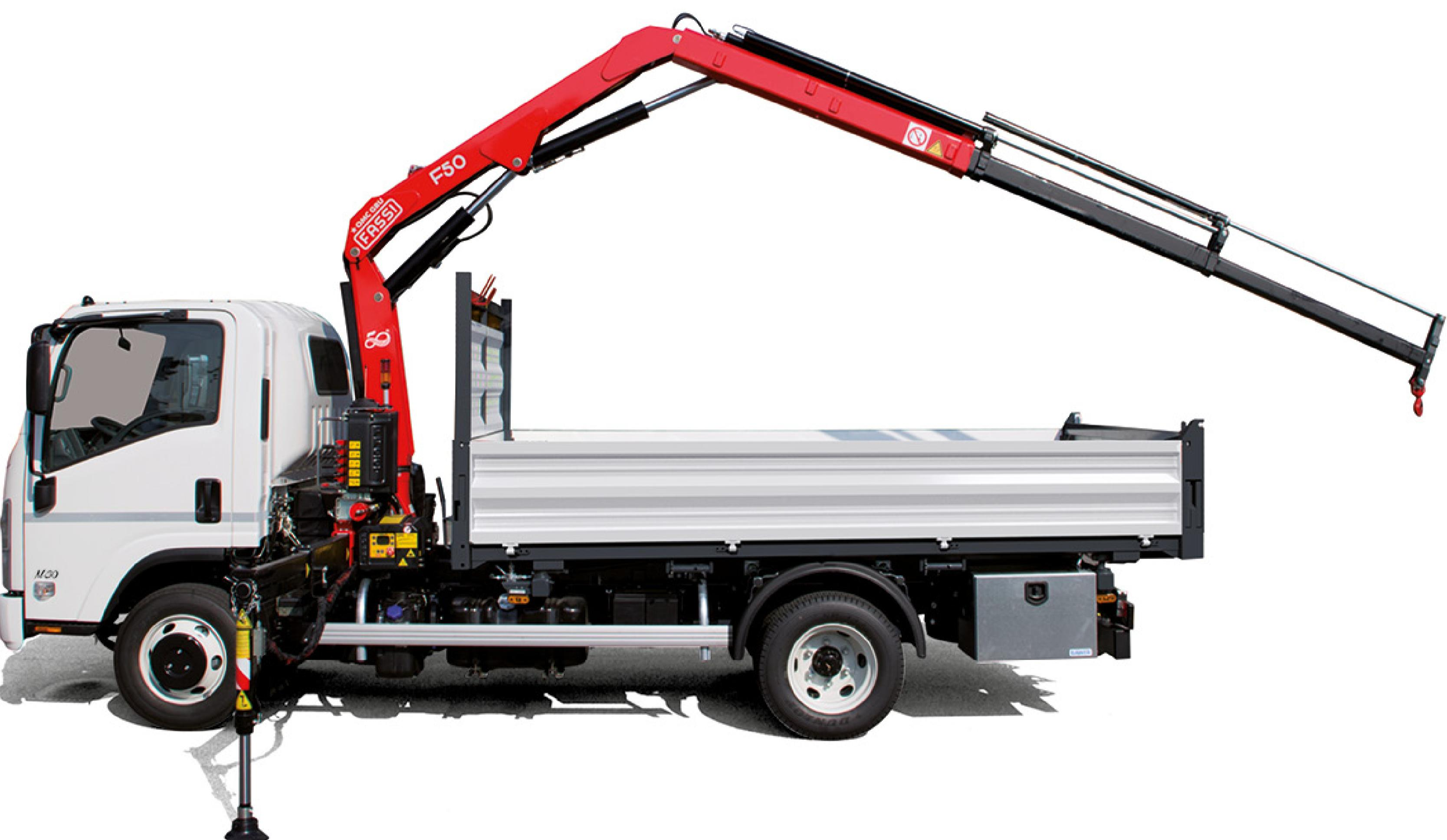
Loading deck structure in S355JR steel th. 4 mm
