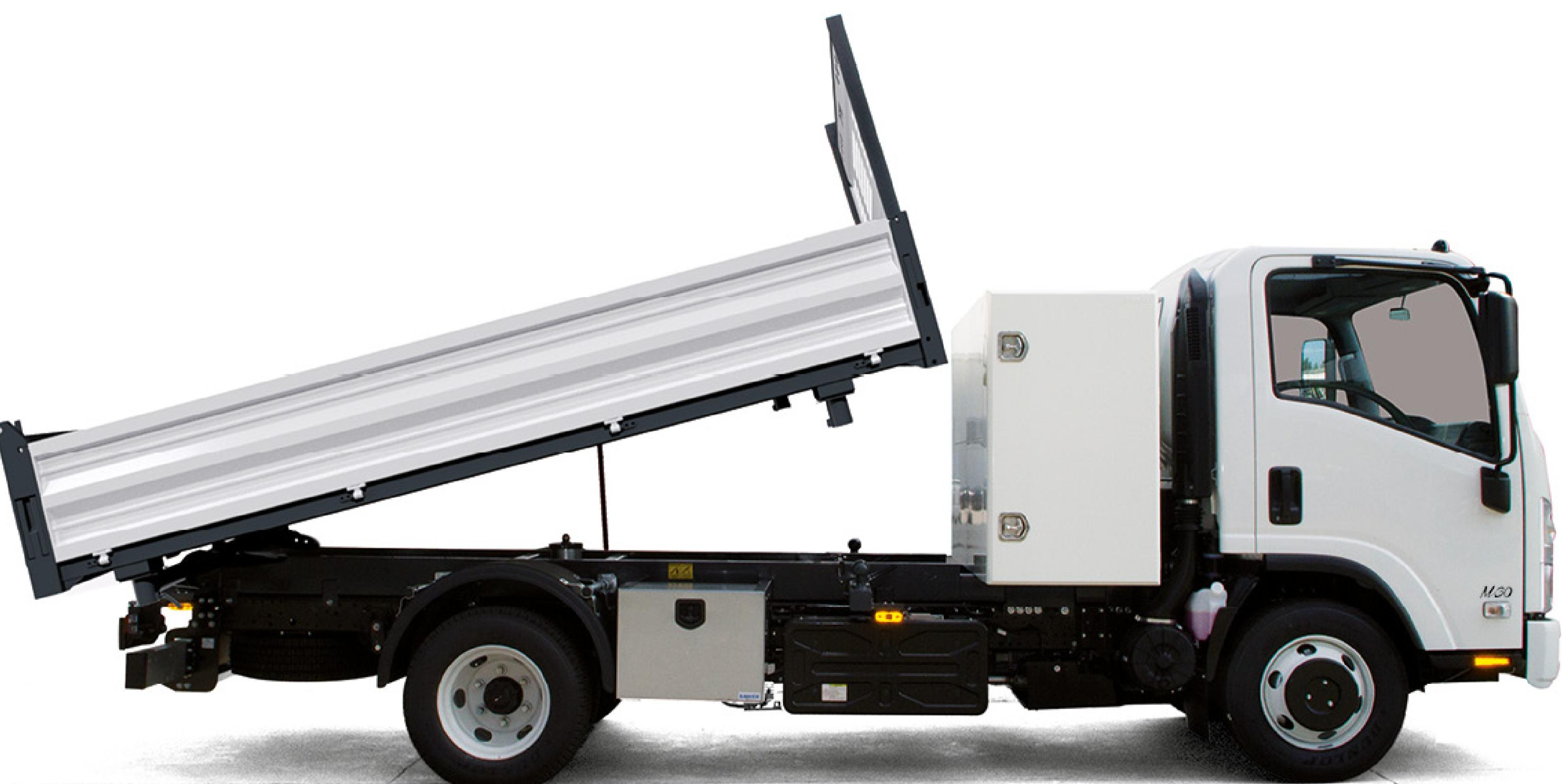
Loading deck structure in S355JR steel th. 4 mm
