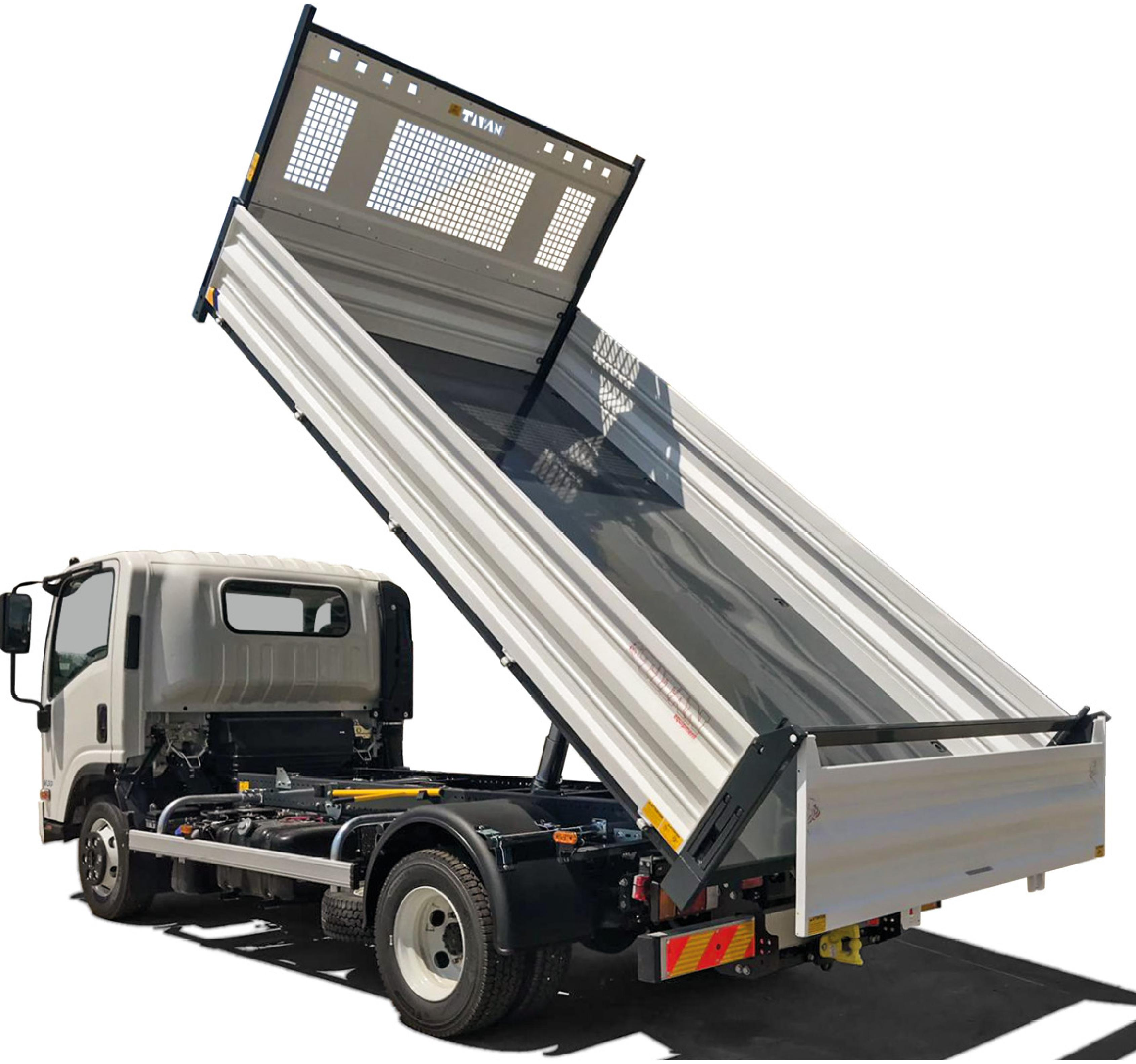
Loading deck structure in S355JR steel th. 4 mm
